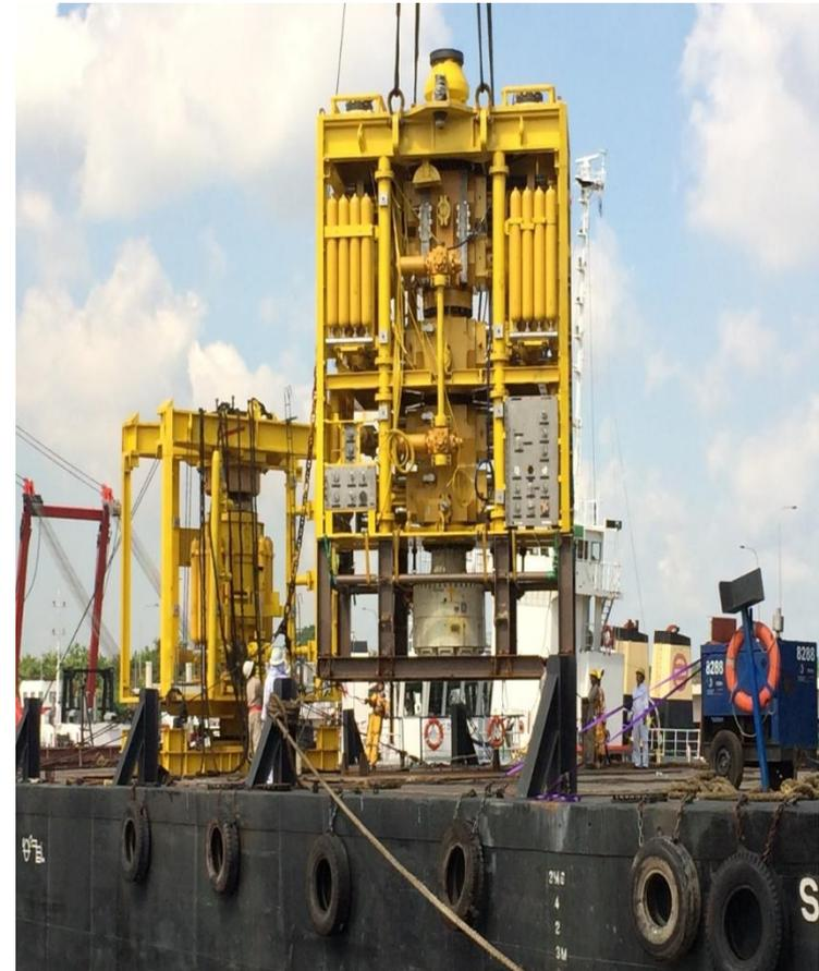
Subsea BOP stack up and barge transportation
