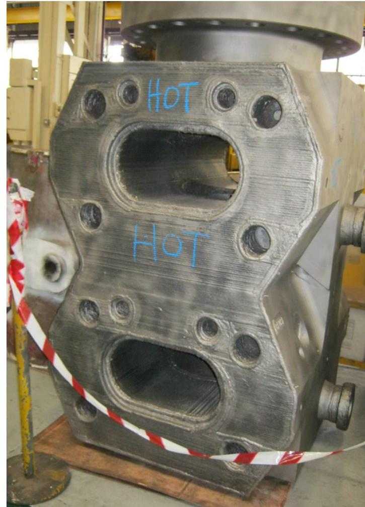
Welding / Cladding and Furnace PWHT
