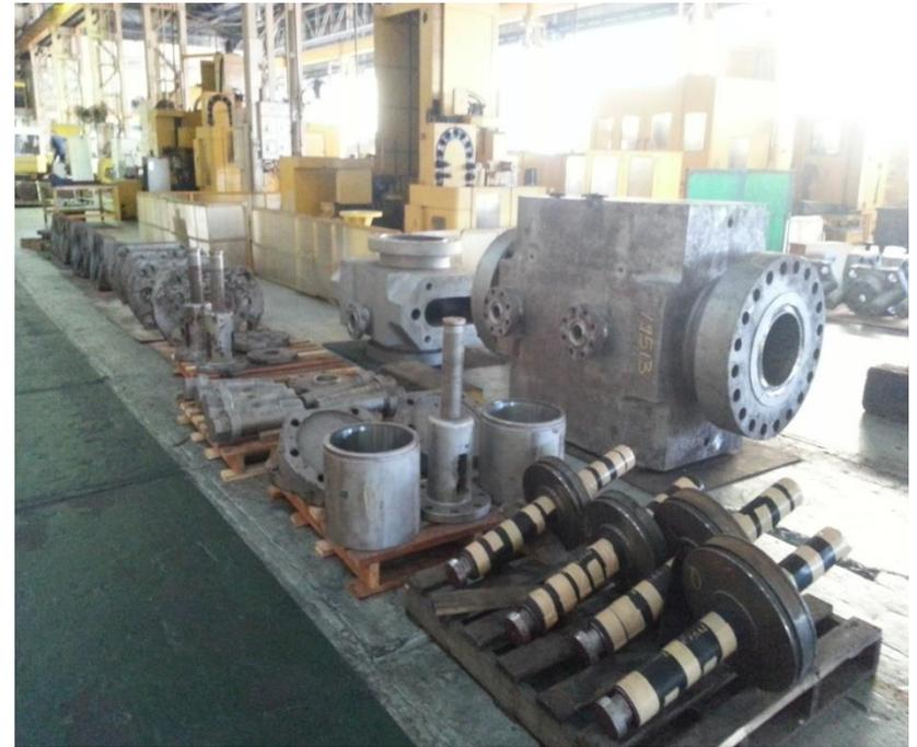
Dismantling and blasting for inspection
