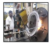
Submerged Arc Welding (SAW)
