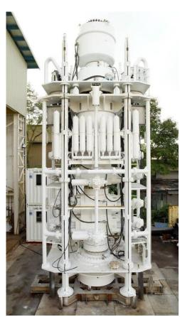
Rebuilt and complete stack-up 18 3/4"
