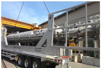
**Managed Pressure Drilling (MPD) equipment**
